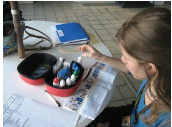
KT LaBadie, an Environmental Health Specialist, testing the water quality parameters of an area pool to ensure a safe swimming environment for the public.
