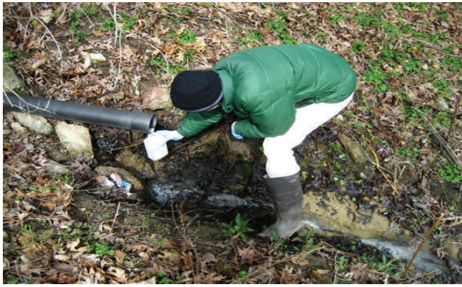
Tamara Ewoldt, an Environmental Health Specialist, samples a discharging wastewater system.
